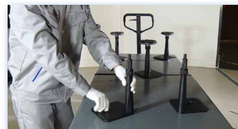
Positioning and fixing components with specialized fixtures
